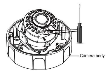
9. Screw back the Set Screw using the supplied Hexagon Wrench.
