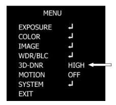
Switch to HIGH, MIDDLE, LOW and OFF to enable or disable noise reduction on dynamic recordings.
